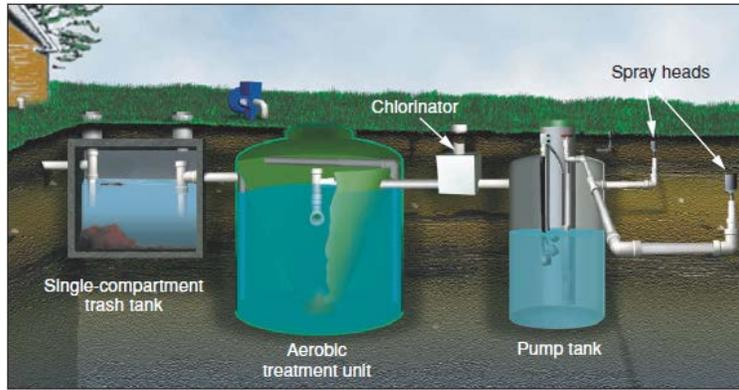
Figure 2: Conceptual drawing of an aerobic treatment unit and spray system.
