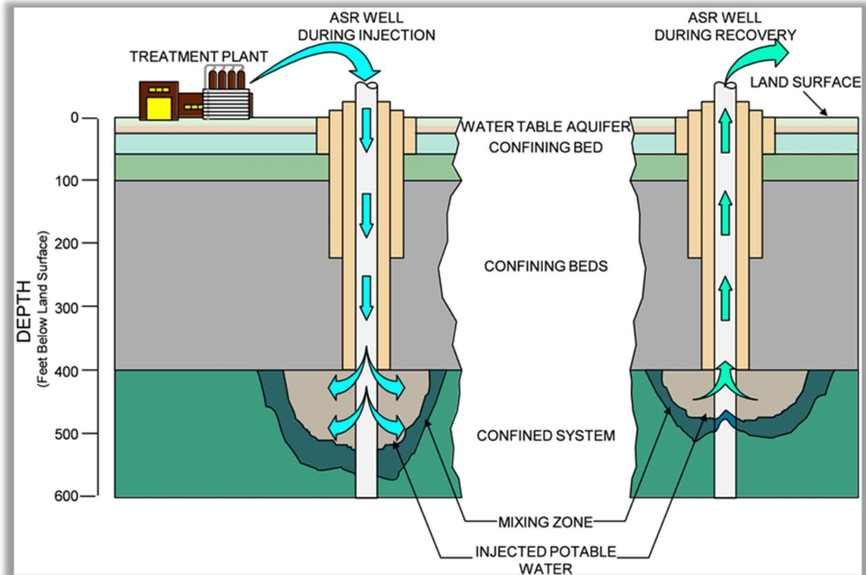
Figure 7. ASR Injection and Recovery (Bloetscher et al., 2014)
