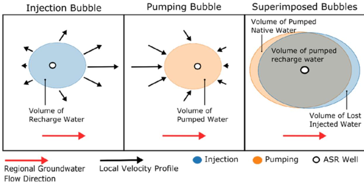
Figure 2. Schematic for Recoverability (Alcalde, 2021)
