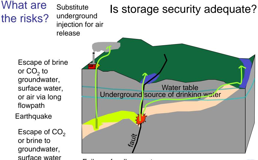
Failure of well cement or casing resulting in leakage
